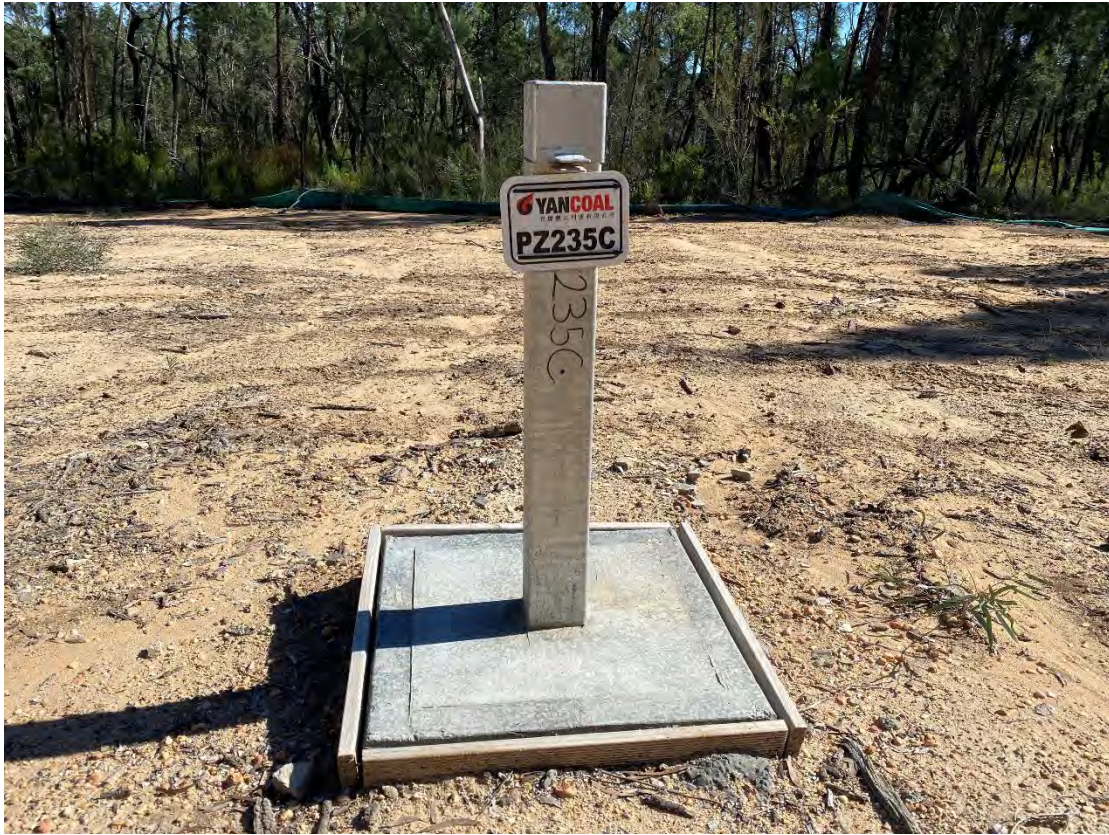
Plate 25 – Piezometer PZ235C - redrilled
