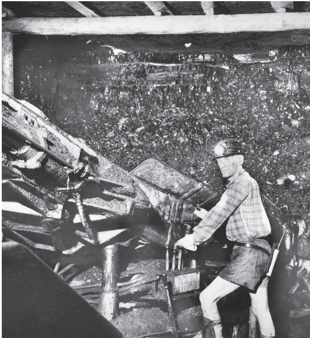
MINERS OPERATING AN ARC WALL COAL CUTTER, TO CUT THE FACE. E STEWART AND T GLEGHORN, NOVEMBER 1957. PHOTO: M. BARRETT COLLECTION
