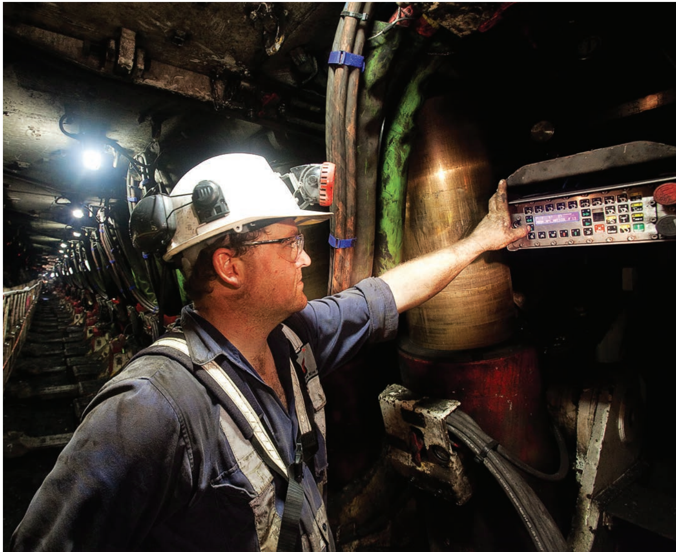
AUSTAR EMPLOYEE GERARD MILES OPERATES THE HYDRAULIC SHIELDS ON THE LONGWALL FACE, 2011. PHOTO: YANCOAL
