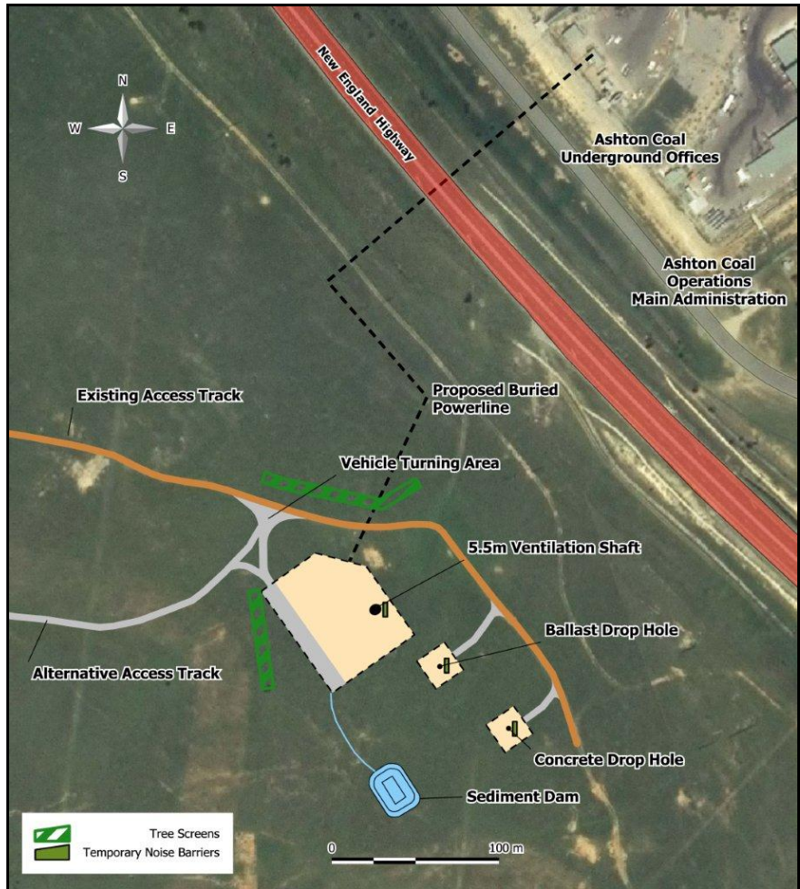
Figure 3. Recommended Temporary Barrier Locations
