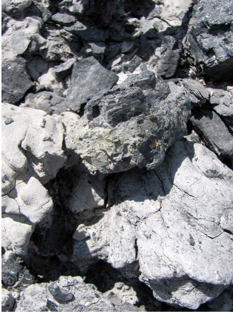
Plate 14: Example of pyritic reject clast from a reject pile in the NEOC overburden dump.
