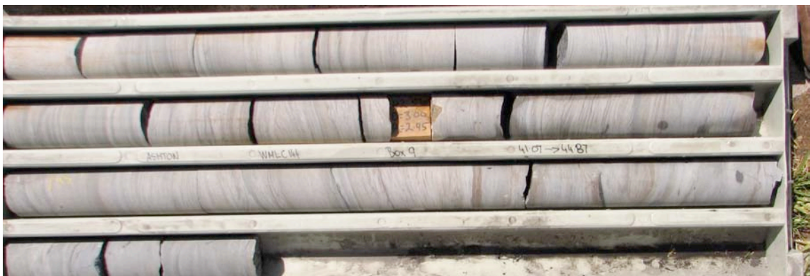
Plate 2: Example of bedded sandstone from hole WMLC144, 41.07-44.87m depth.
