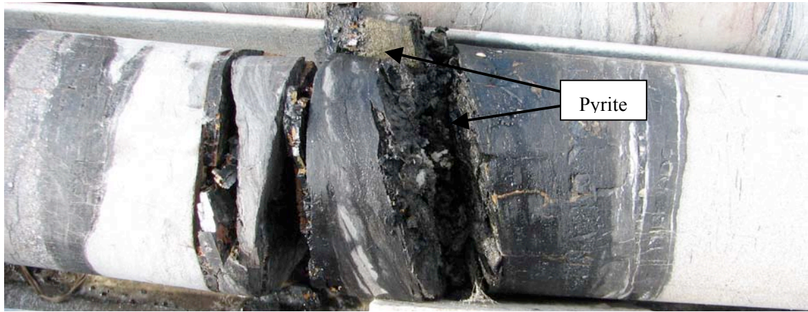
Plate 9: Pyrite vein in carbonaceous mudstone/coal from hole WMLC007, 66.90m depth.
