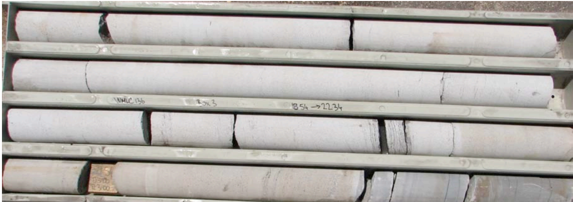
Plate 1: Example of semi-massive sandstone from hole WMLC144, 18.54-22.34m depth.
