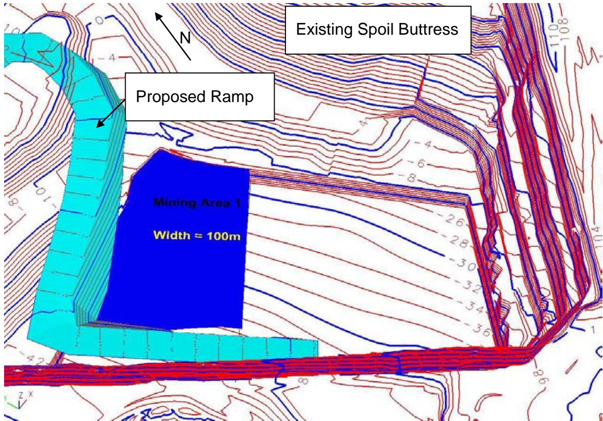
Figure 8 First mining area with ramp
