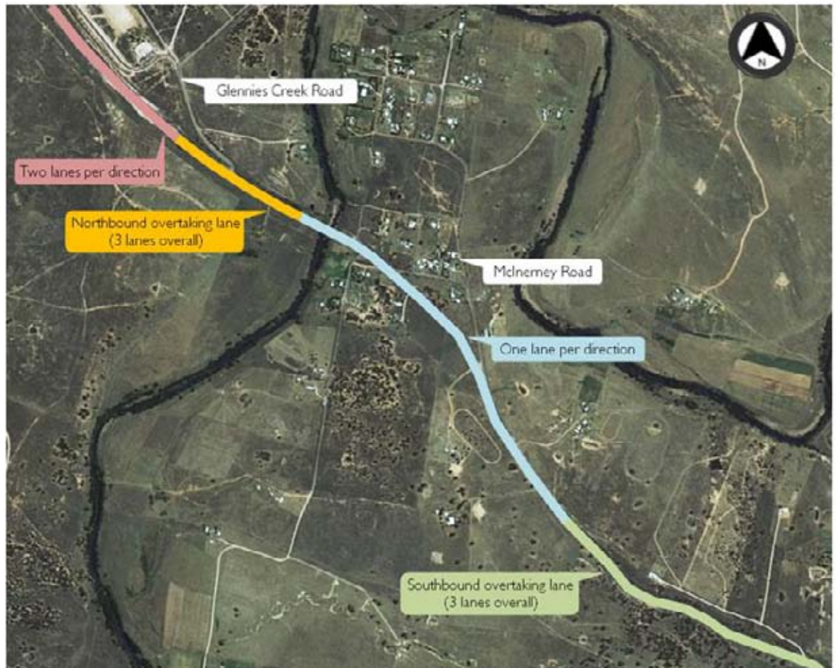
■ Figure 3-2 Lane Configuration on New England Highway
