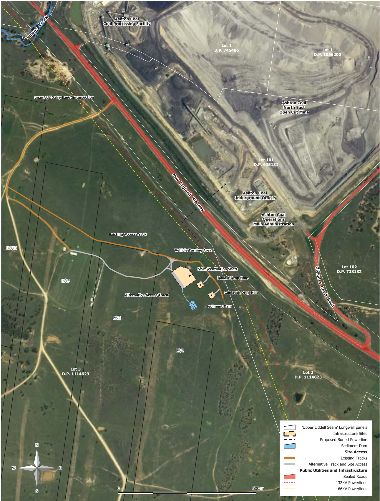
Figure 1: Proposed position of ventilation shaft and drop holes, and associated infrastructure pads (Source: Wells Environmental Services)
