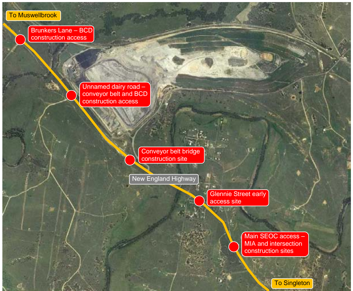
■ Figure 4.2: Location of adjacent potentially concurrent worksites
