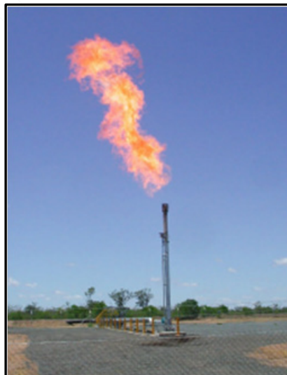
Figure 3: Open “candlestick” flare in operation
