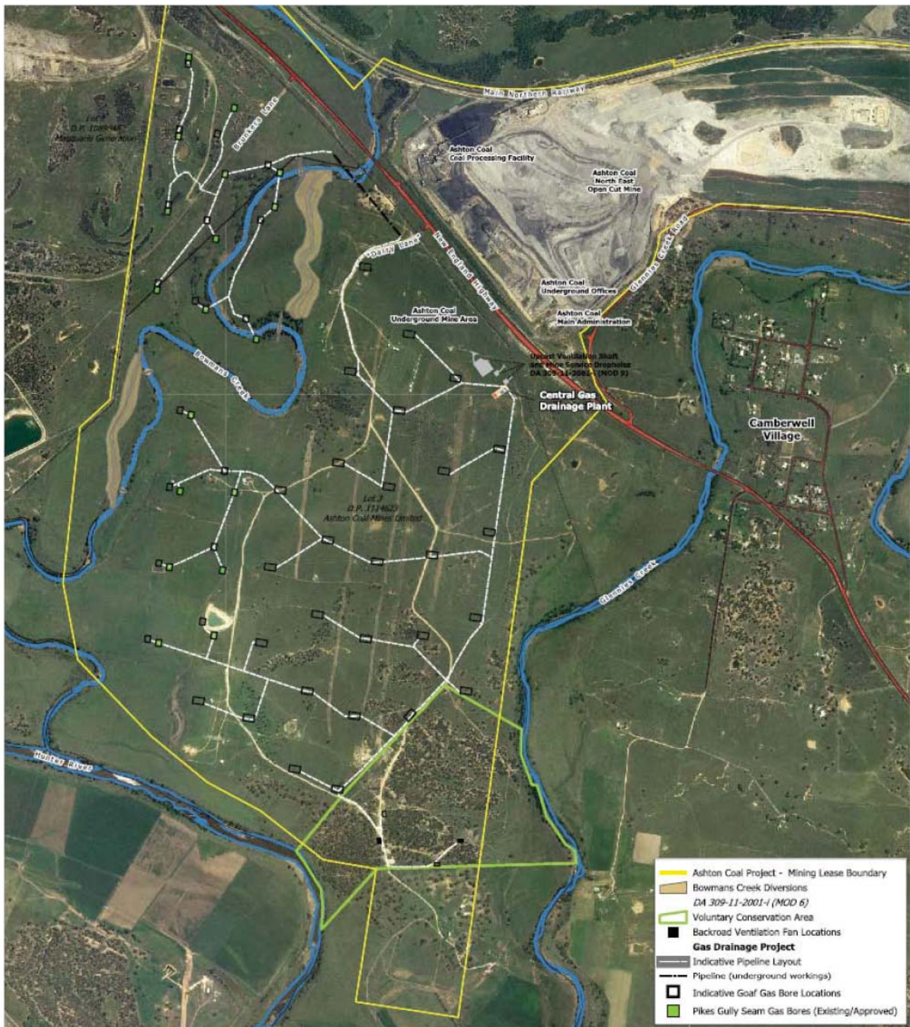
Figure 4: Indicative layout of proposed surface gas reticulation pipeline
