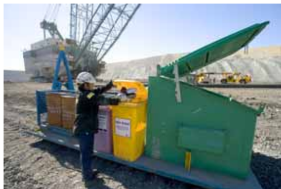
A typical skid-mounted waste handling unit
