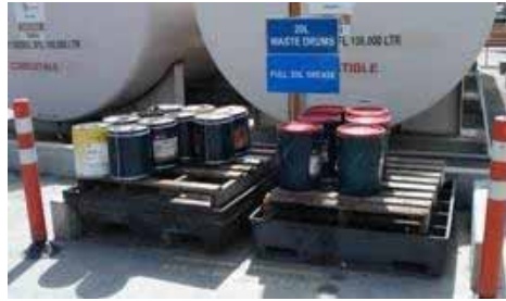
Used drums stored in bunded areas prior to collection and disposal
