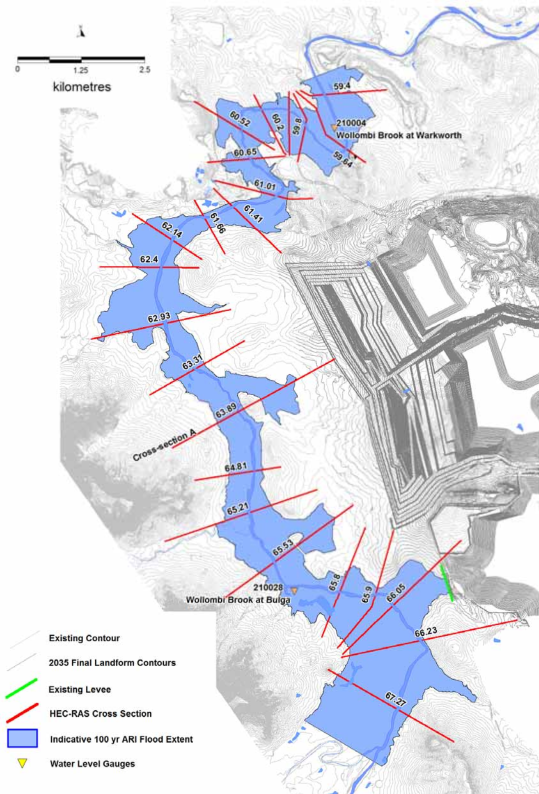
Figure 5.2 HEC-RAS Model Configuration and 100 Year ARI Design Flood Extent
