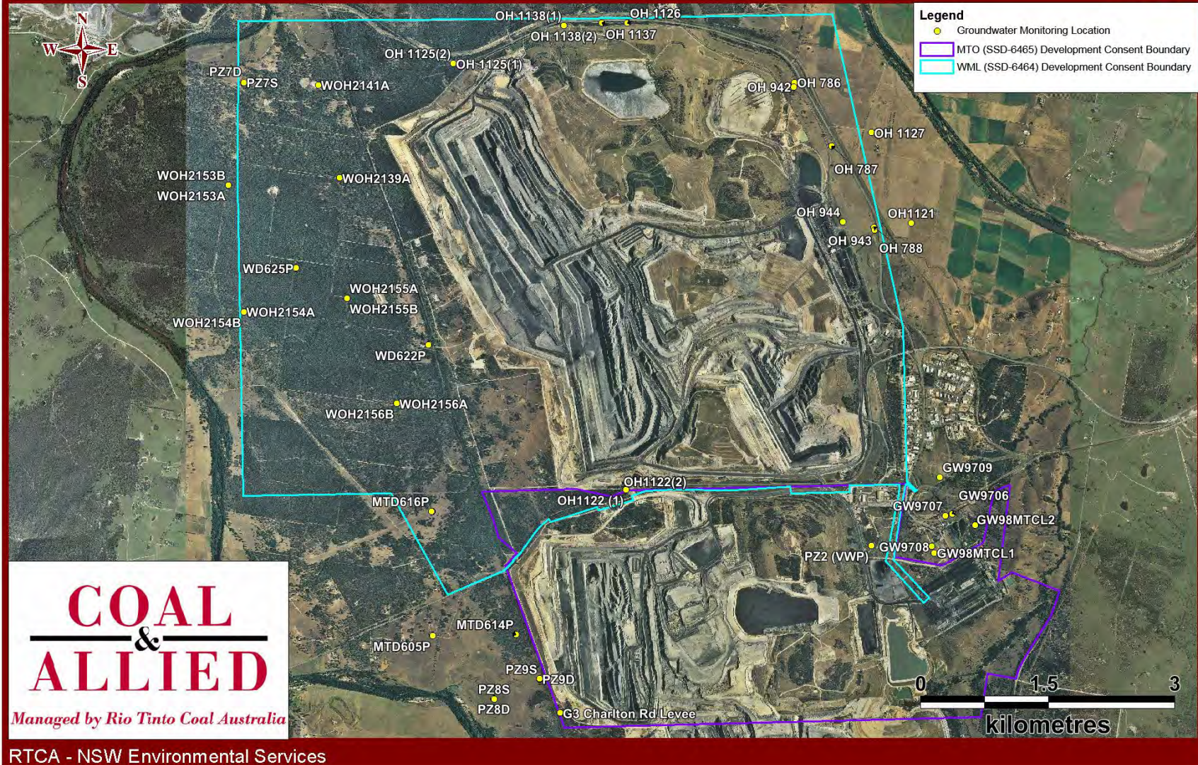
Figure 59: Groundwater Monitoring Location Plan
