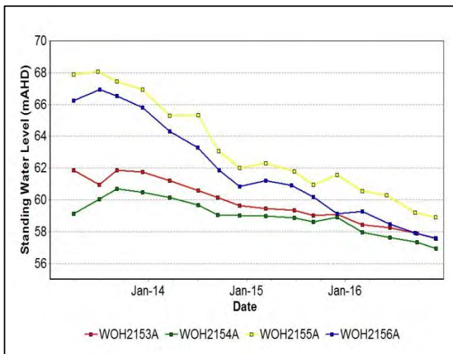
Figure 27: Redbank Seam Standing Water Level - December 2016
