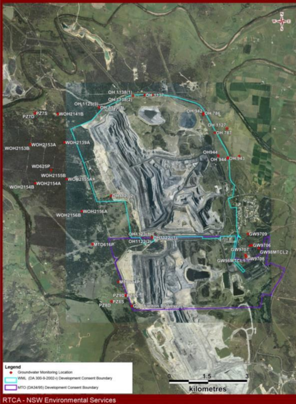
Figure 49: Groundwater Monitoring Location Plan
