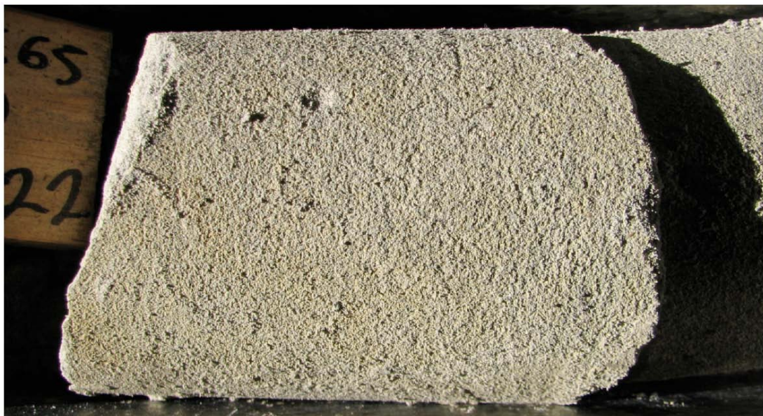
Plate I-4: Jarosite and sulphate salts in sandstone, indicating fine disseminated pyrite. No obvious carbonaceous material or pyrite. Hole WC218C, 17.22m.
