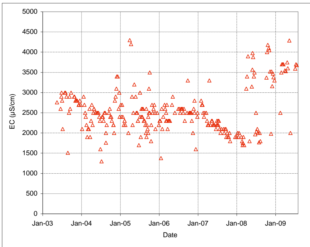
Figure I-41: Results of EC monitoring of the Duralie Coal Mine pit sump (SW4).
