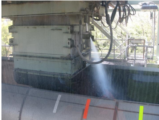
(a) Loading coal to wagon from Duralie Coal Mine Loadingout and application of water to coal surface
