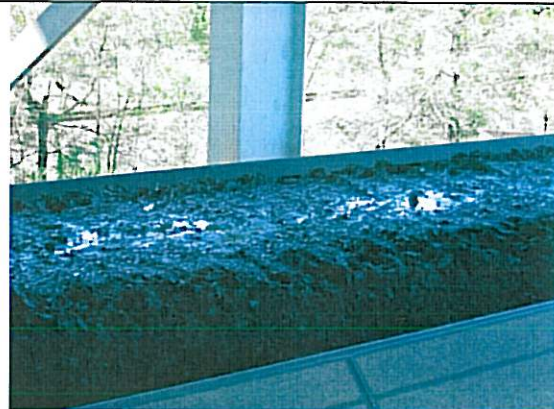
Plate 3: Ponding of water on coal surface indicating high wetting level following water spraying during loading
