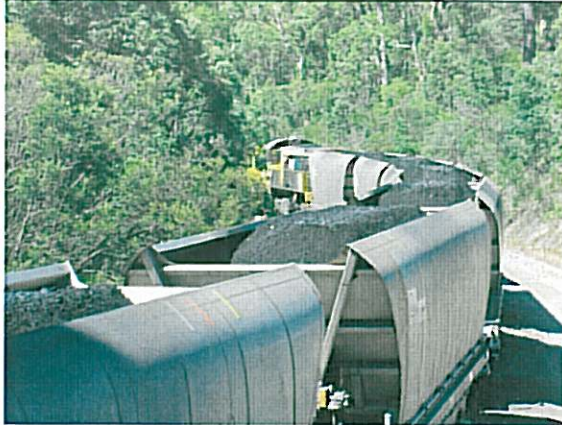
Plate 1: Wagons loaded with coal from the Duralie Coal Mine with surface profile slightly above the sill of the wagon
