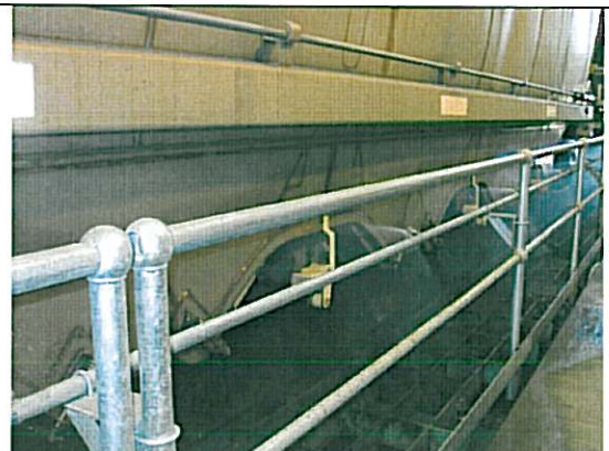
Plate 4: Coal unloading at the Stratford Coal Mine with misting sprays and no dust emission observed
