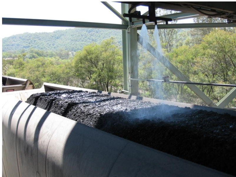
(b) Re-wetting of coal surface before departure of coal train from Duralie Coal Mine
