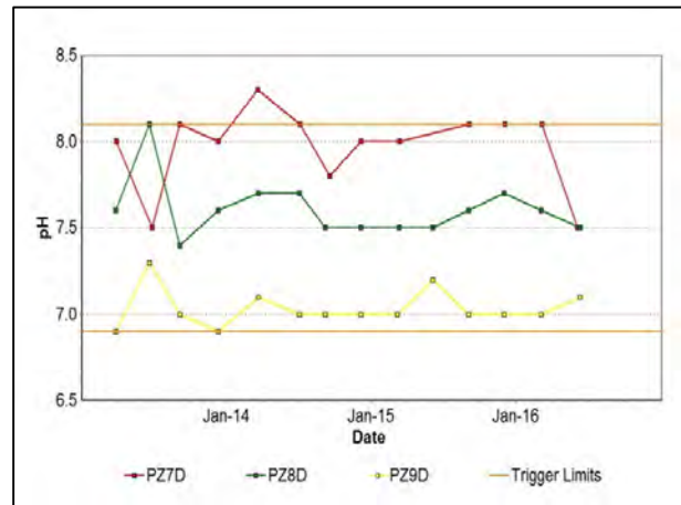
Figure 29: Shallow Overburden Seam pH Trend - June 2016
