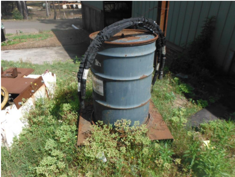
Photo 5 Tank not within bunded area
