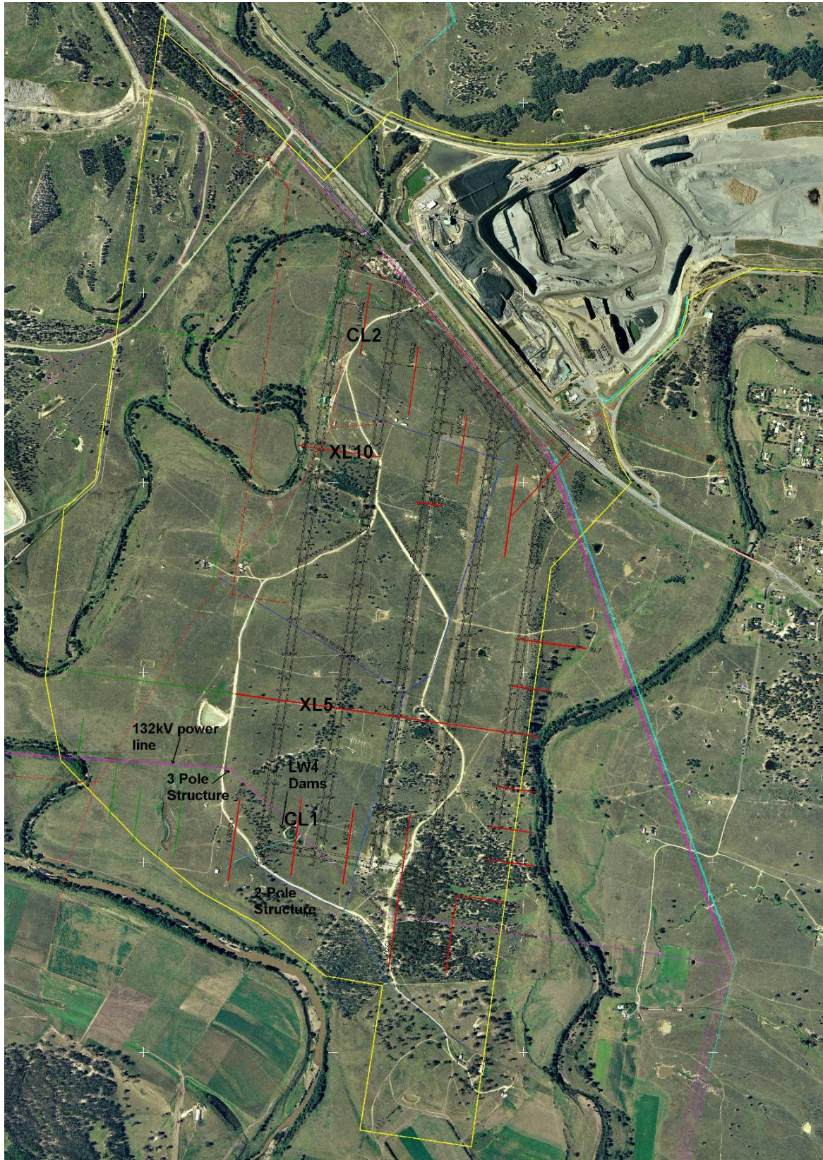
Figure 2: Plan location of Monitoring Cross Lines. Also shown is the 132kV power line and longwall 4 dams.
