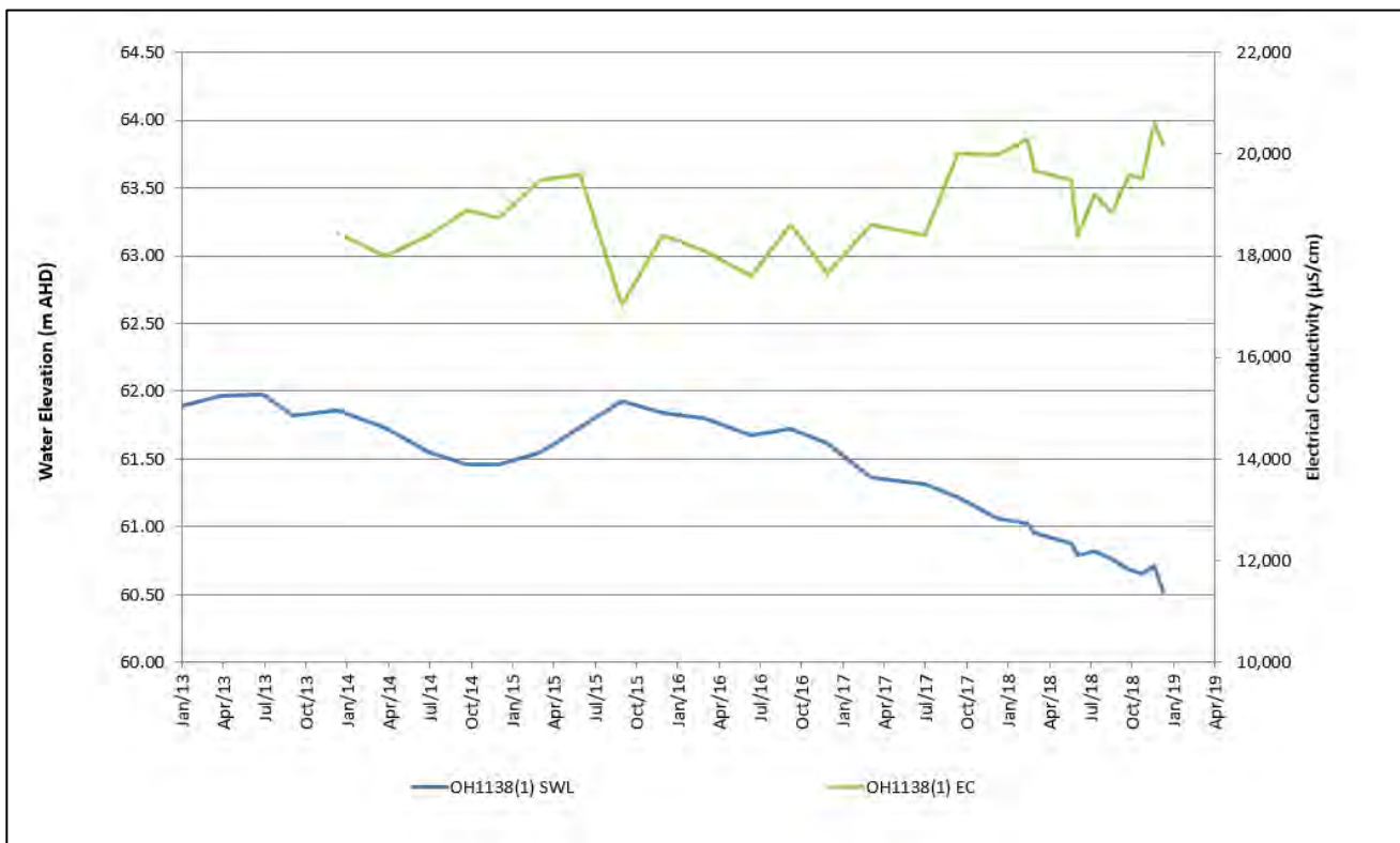
Figure 5-23 Electrical Conductivity and SWL Trends at OH1138(1)
