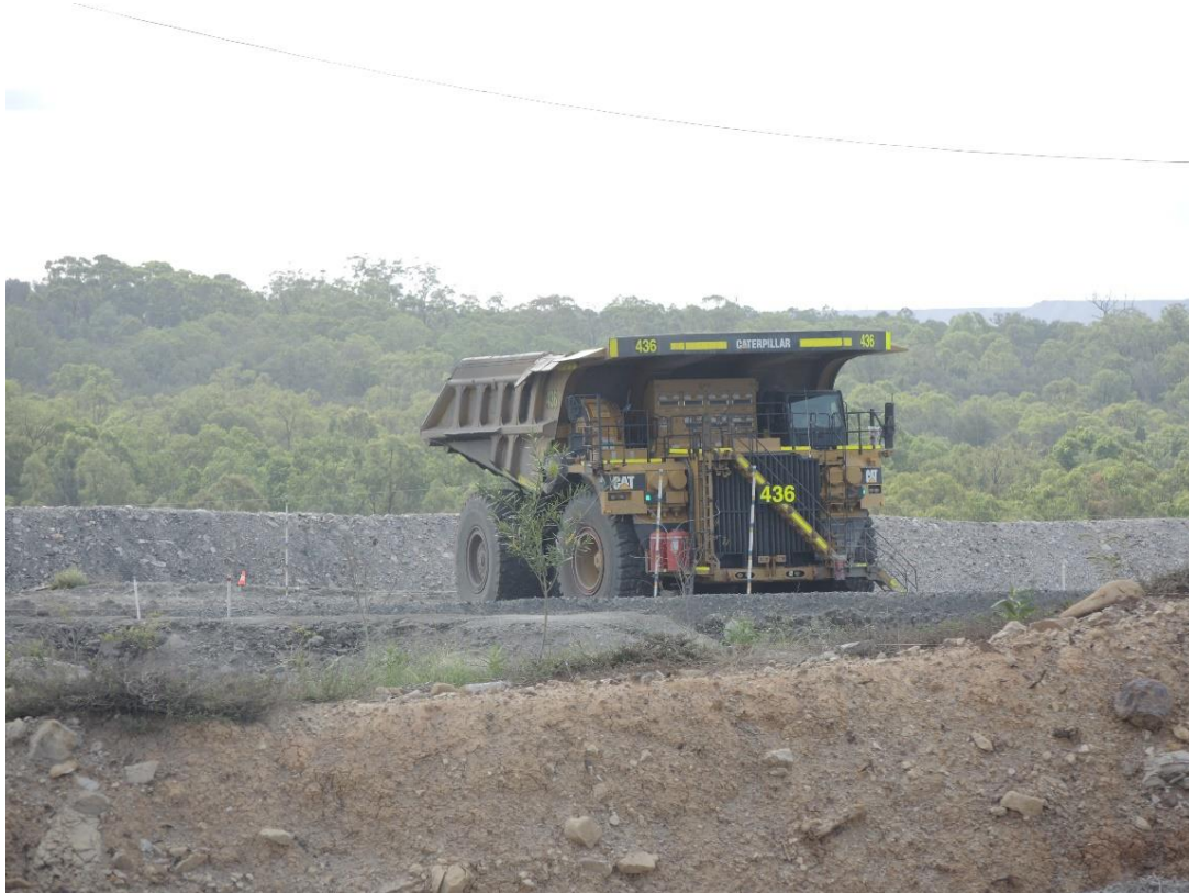
Plate 9 Operating mobile plant fitted with noise attenuation (front grill panel)
